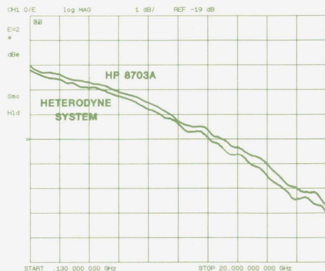
Fig. 4. Measurements of a reference receiver with the HP standards laboratory's heterodyne YAG system and with an HP 8703A.
